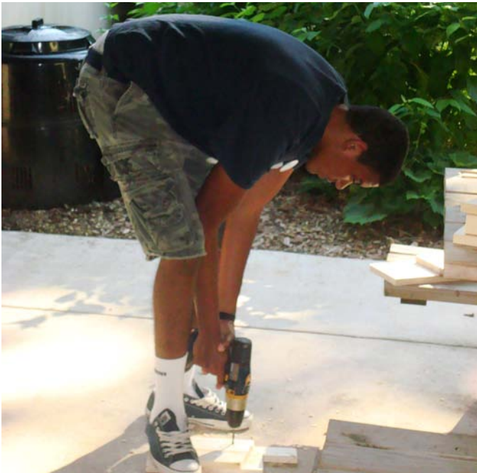
Malcolm creates pilot holes on one of the sides of his birdhouse.
